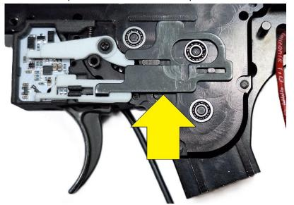
8. At this point you can insert the gearbox into receiver and assemble the replica, but we recommend on adjusting the trigger feel. It can only be done while the gearbox is outside of the replica. Instruction on how to do it is available below. Do not forget to also perform selector calibration before connecting the motor for final assembly, details of which are also described in further chapters of this manual.
