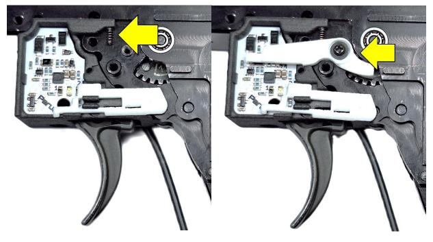
7. Insert original metal selector plate into the white selector part.
